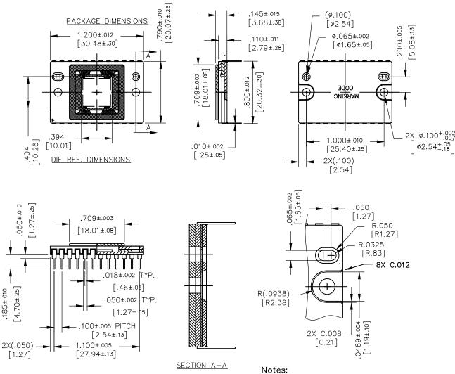
Cover glass is manually placed and visually aligned over die – Location accuracy is not guaranteed.
