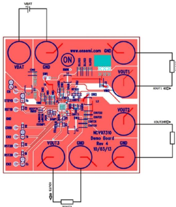
Figure 1: NCV97311MW33AGEVB Board Connections
