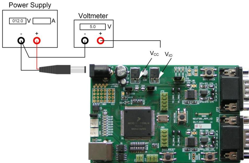
1. Set the boards to default configuration according to Jumpers and Default Configuration section.
