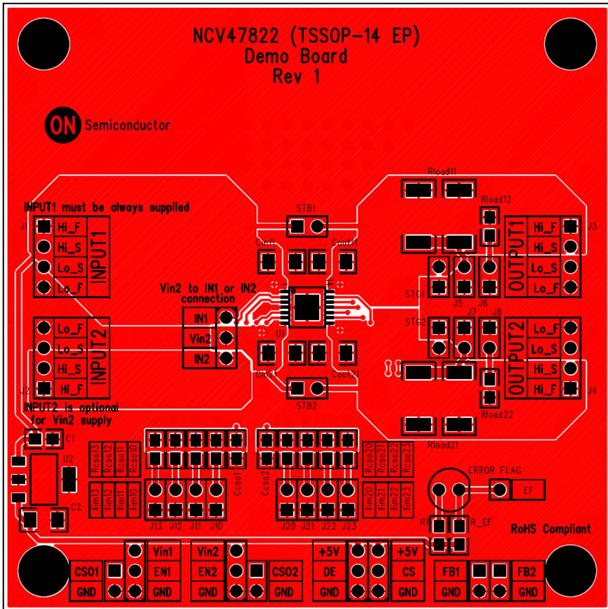
Figure 2. Top side PCB Layout (3 x 3 inch)
