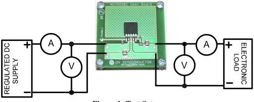
**Figure 1: Test Setup**
