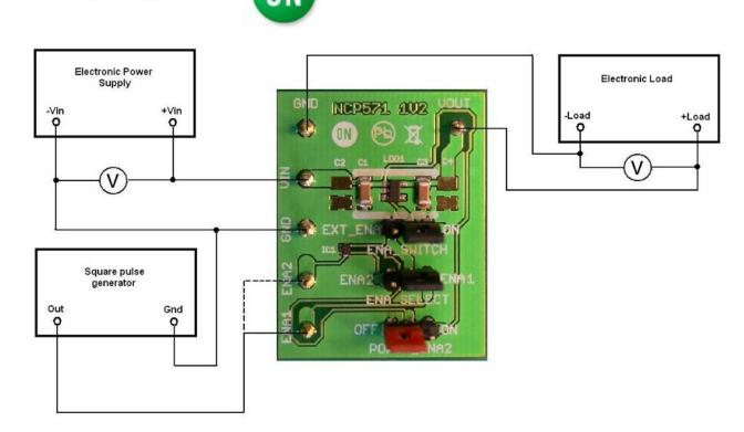
1. Enable pin connected to Vin
