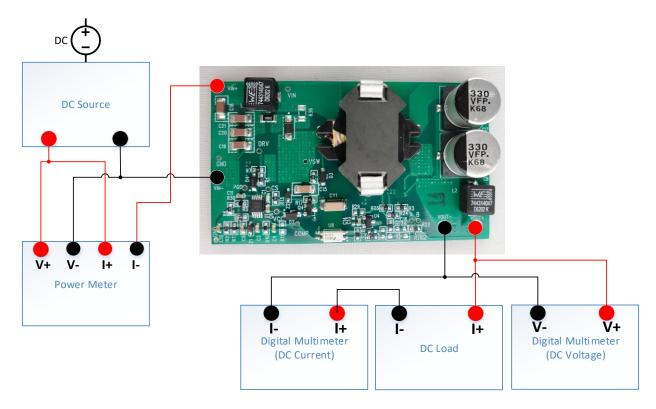
Figure 1 - Test Configuration
