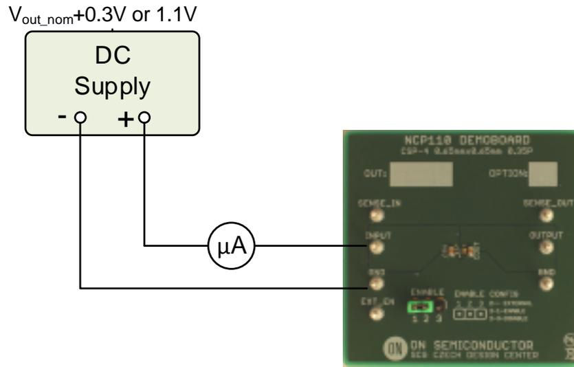
Figure 1: Test configuration for measurement  $I_Q$ , Quiescent Current
