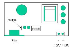
Figure 1 Top view of NCP1013 demo board, marked MIC1782
