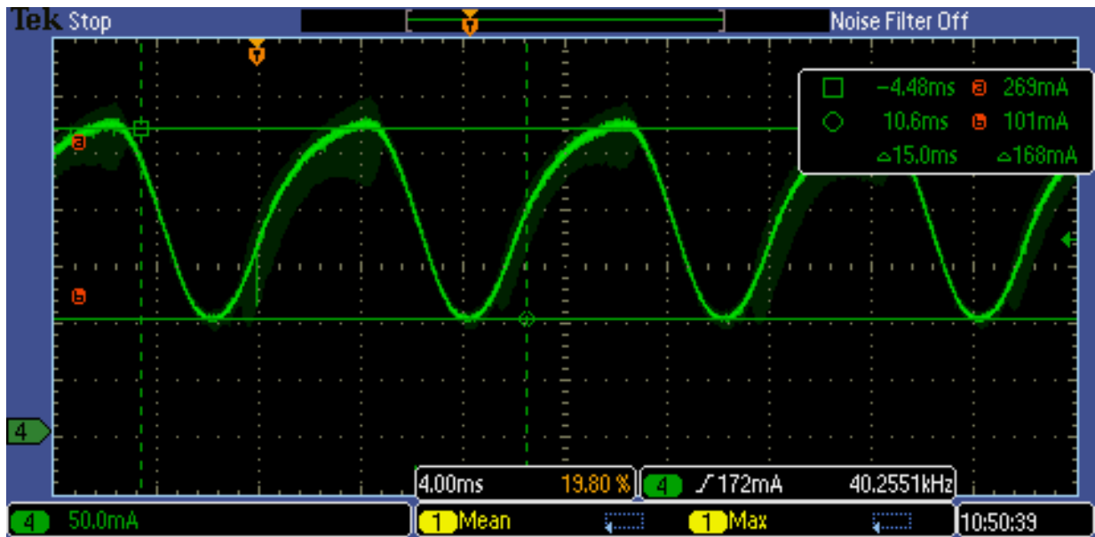
Figure 11. Output Ripple 75% Pk - Pk
