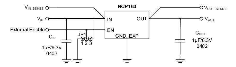
The NCP163 is 250mA high performance LDO with low quiescent current ( $12\mu A$  typ.) and very high PSRR. The NCP163 also offers excellent load/line transients and ultra-low noise.
