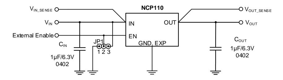
The NCP110 is 200mA low  $V_{IN}$ , low noise, high performance LDO with low quiescent current (25 $\mu$ A max.) and very high PSRR. The NCP110 also offers excellent load/line transients and ultra-low noise.
