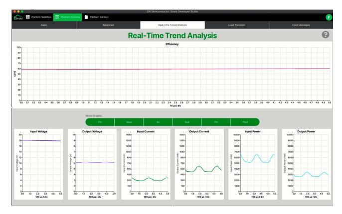
5. The load is controlled from the GUI: We don't need an external electronic load. Please note, only power supply is required.
