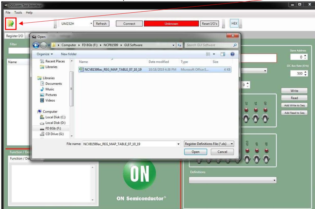
5. Once the register map loaded, click “connect” to establish communication with the I<sup>2</sup>C dongle. “Unknown” field will turn from red to green with “FT\_OK” see below.
