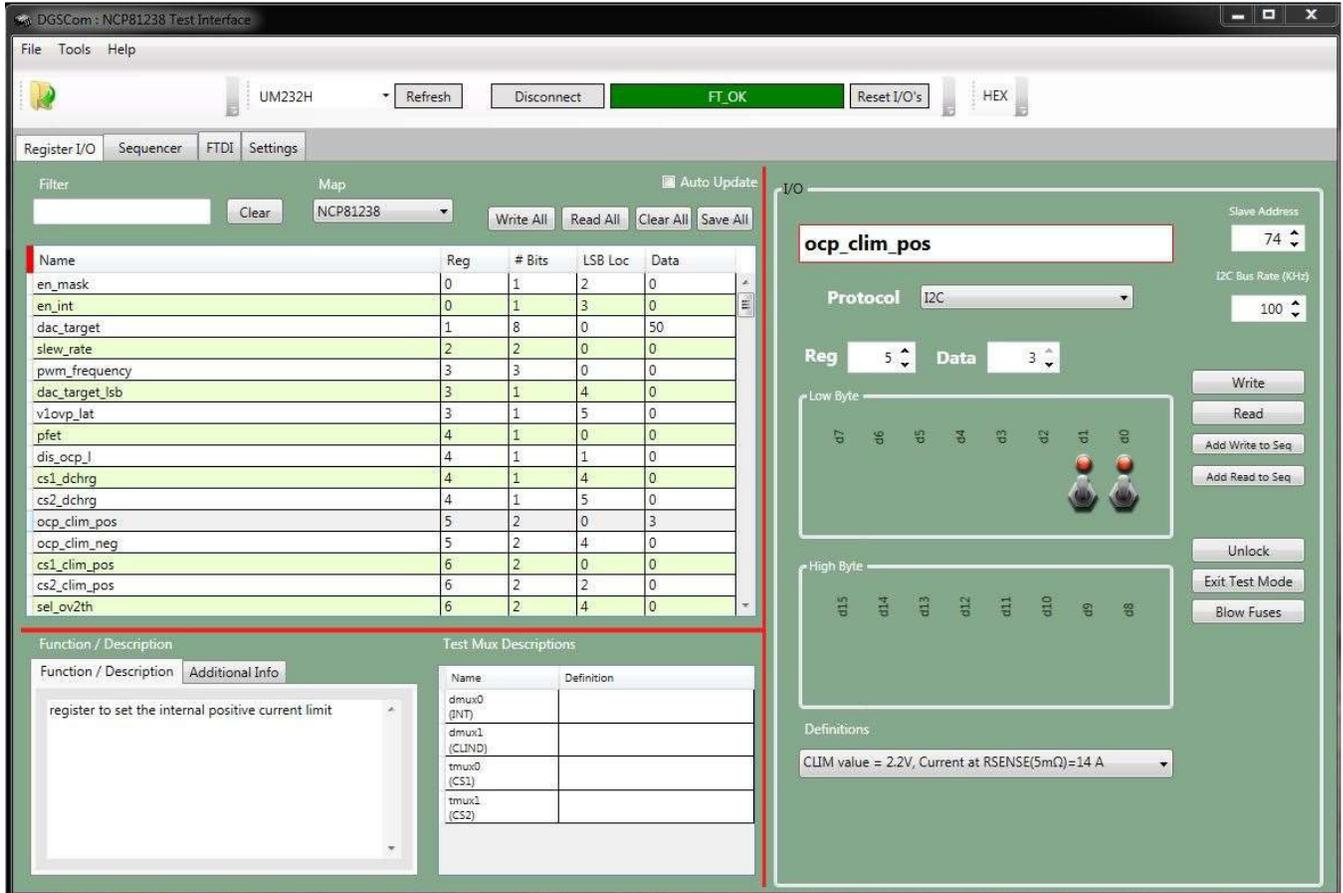
10. As you can see, there are many read/writable registers. They can all be changed to accomplish different things. In the data package is a complete register map (NCP81599\_register\_map\_rev3.pdf) with register definitions. Use that as a guide to change any register values.
