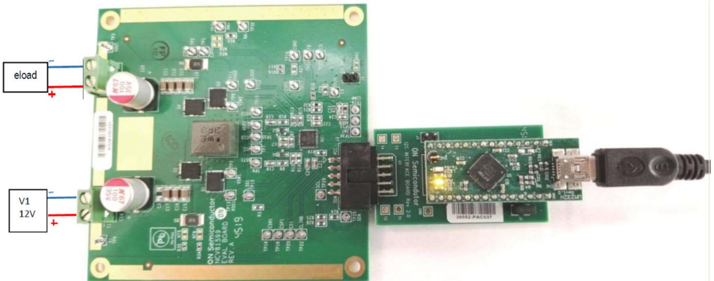
Note: The reason for the two pin header connected to the bottom of the board, rather than on the C7 pads is due to the fact that the C7 pad is before the output pi filter, which is used to suppress high frequency noise on the output, the two pin header can be used with a differential probe. You can also use a passive probe to observe the output by probing the test point on the Q6 drain pad.
