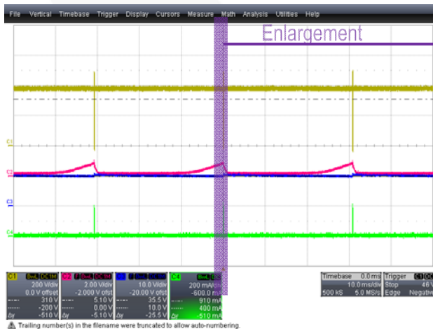
Figure 15. No-Load Condition, 265V AC , (CH1: V DS (200V/div), CH2: V FB (2V/div), CH3: V CC (10V/div), CH4: I DS (200mA/div), Time: 10ms/div
