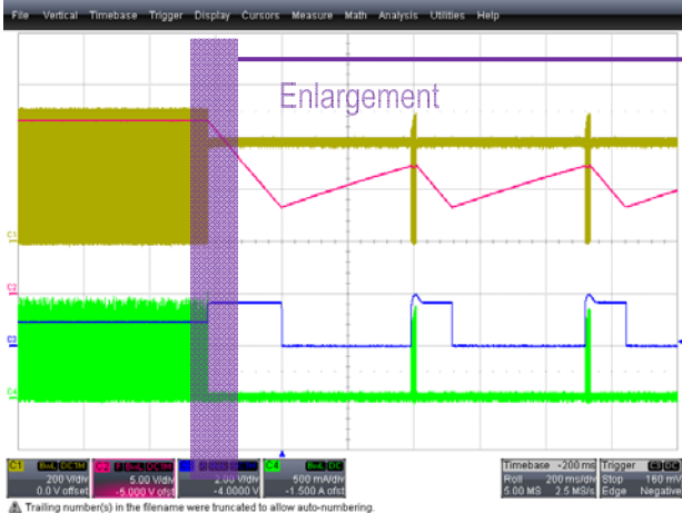
Figure 31. OSP Triggered: V_{FB} = 1.60V , 5V Output Short with 265V AC and Full-Load, CH1: V_{DS} (200V/div), CH2: V_{CC} (5V/div), CH3: V_{FB} (2V/div), CH4: I_{DS} (500mA/div), Time: 200ms/div and 10ms/div
