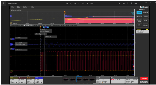
Figure 19. Startup @ 50 V/3 A
