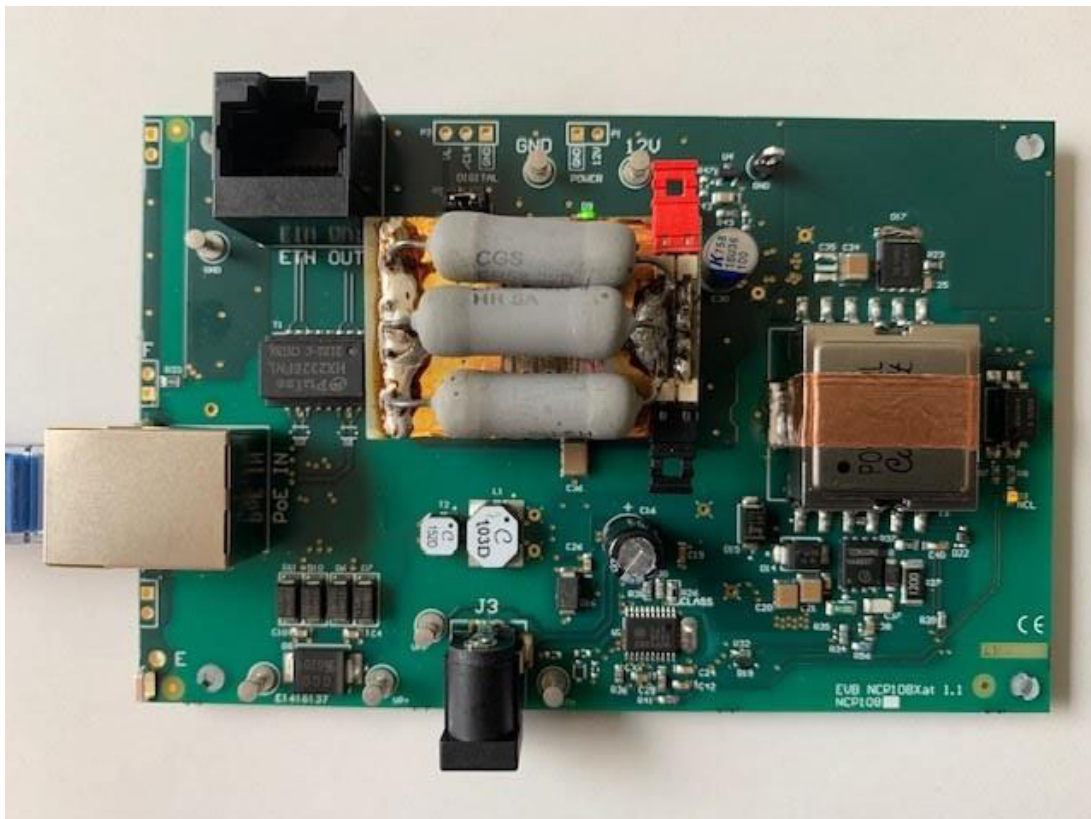
Figure 13. Emission Test DUT: NCP1083REF12VGEVB with 7.3 \Omega Load
