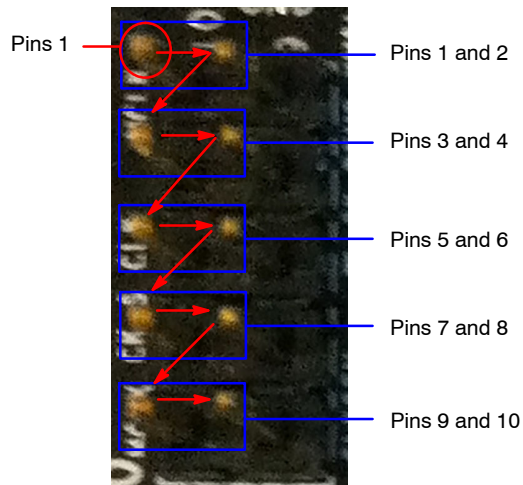
Figure 6. Pin Locations and Assignment of Grouped Jumpers; Pin 1 is Located at the Top-Left Corner and Increases in a Zigzag Fashion Shown in the Picture
