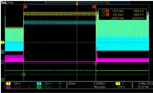
Figure 24. 115 Vac to 230 Vac at 20 V 5 A (CH1: Vin-rect, CH2: Vds-pfc, CH3: Vcs-pfc, CH4: Vcc-pfc)
