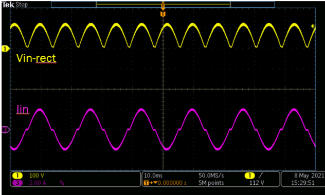
Figure 20. 90 Vac & 20 V 5 A (CH1: Vin-rect, CH3: lin)
