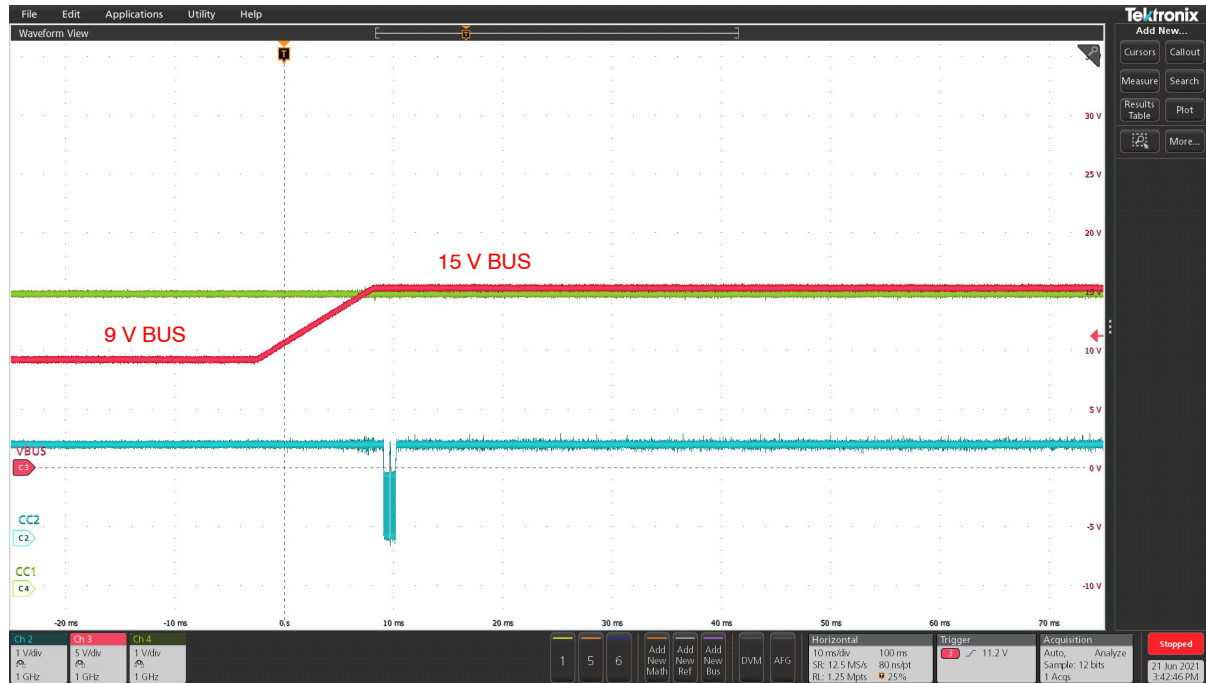
Figure 7. Sink Request 15 V PDO, CC = CC2, VCONN = CC1
