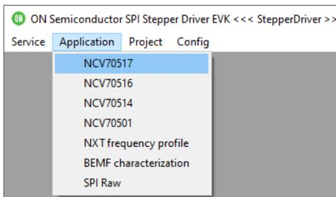
There is a possibility to use low level access where each bit in SPI frame can be controlled via “SPI Raw” panel. This allows to create non-standard frames for testing purposes (e.g. with corrupted parity).
