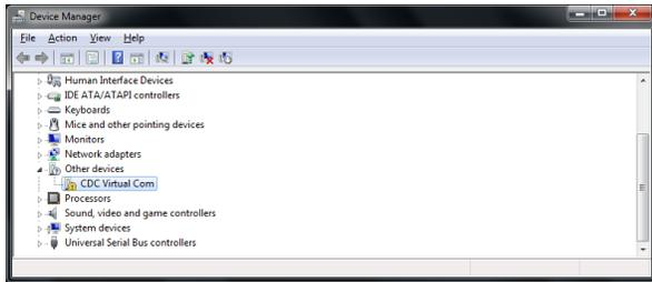
5. Update Driver of not correctly installed device "CDC Virtual Com" by Right button click and select "Update Driver Software"
