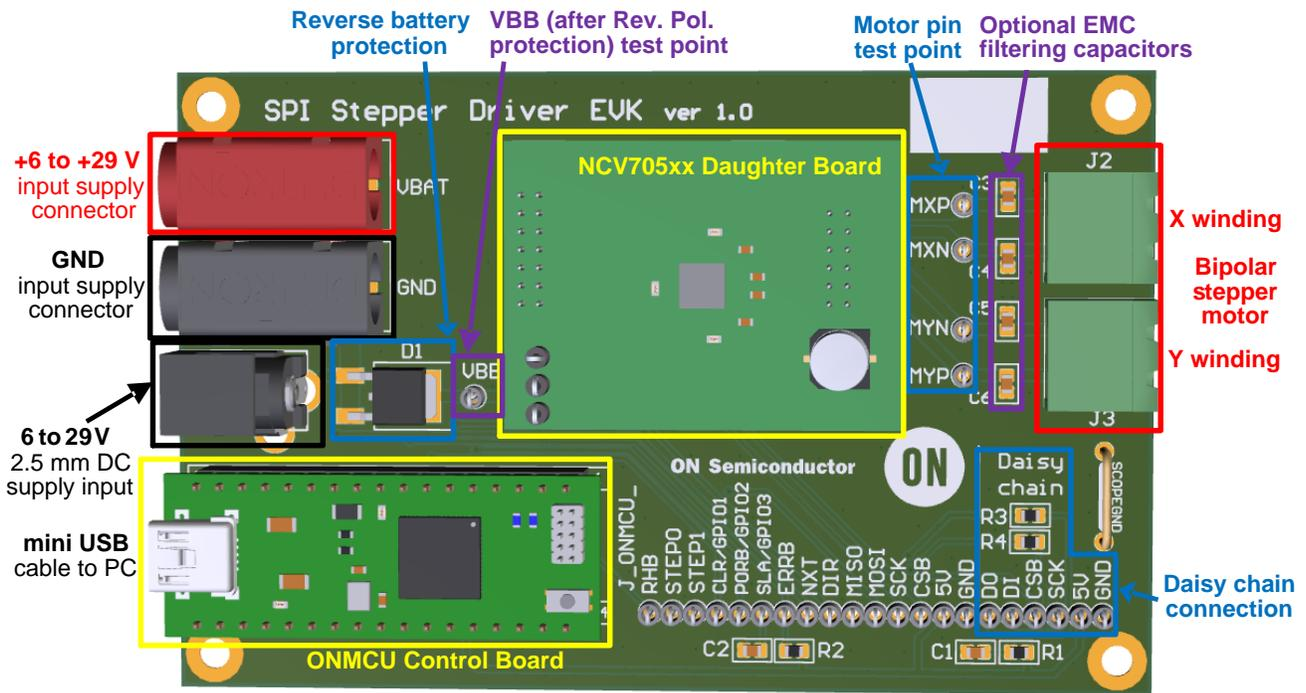
Figure 2. NCV705XXGEVK Micro-stepping Motor Driver Evaluation Board Picture
