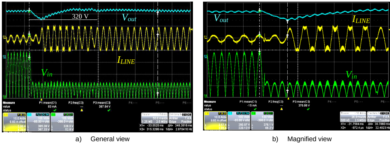
Figure 14. 265 V rms to 90 V rms Line Drop at Full Load
