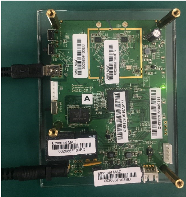
Figure 5. LED Indication When QHS952-DS1-GEVK Powers Up
