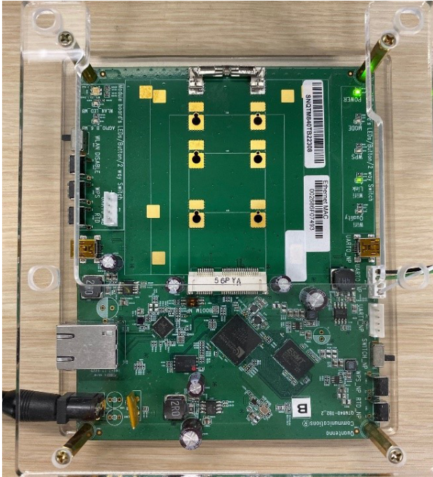
Figure 5. LED Indication When QTM840-TB2-GEVK Powers Up
