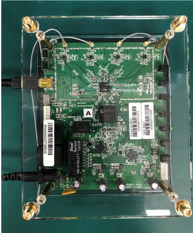
Figure 5. LED Indication When QHS840-5S3-GEVK Powers Up
