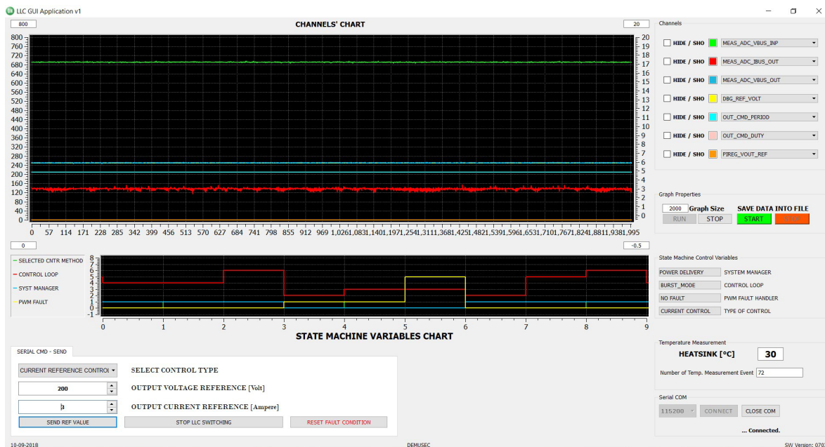
Figure 23. Operation Point : 250 V Voltage Bus and 3 A for Load
