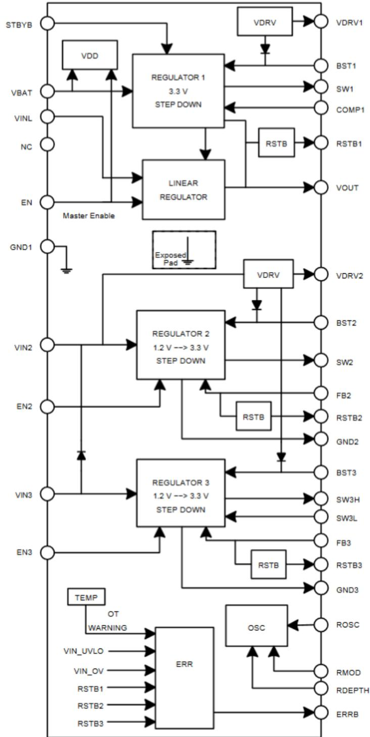
Figure 2. NCV97311A Block Diagram
