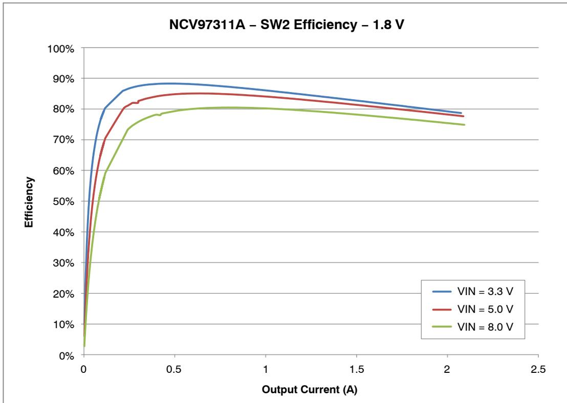
Figure 7. Efficiency for SW2 with a 1.8 V Output
