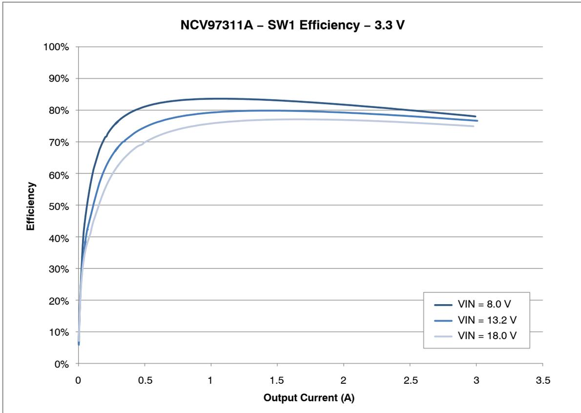
Figure 6. Efficiency for SW1 with a 3.3 V Output
