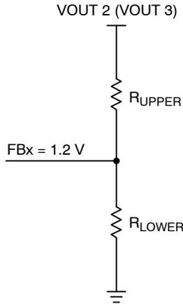
The upper resistor is set to 10 kΩ and is part of the feedback loop. To maintain stability over all conditions, it is recommended to change the only the lower feedback resistor to set the output voltage. Use the following equation:
