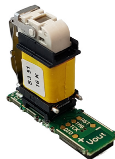
Figure 8. Switch Reference Design without the Wings
