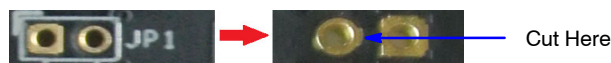
Figure 7. Top and Bottom View of Shorted Jumper. The Bottom View Shows the Trace Location to Cut for Current Measurement
