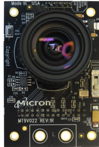
Figure 1. MT9V022 Evaluation Board
