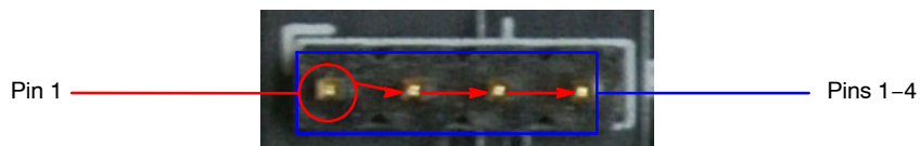
Figure 5. Pin Locations for a Single Jumper. Pin 1 is Located at the Leftmost Side and Increases as it Moves to the Right
