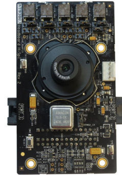
Figure 1. MT9J003 Evaluation Board
