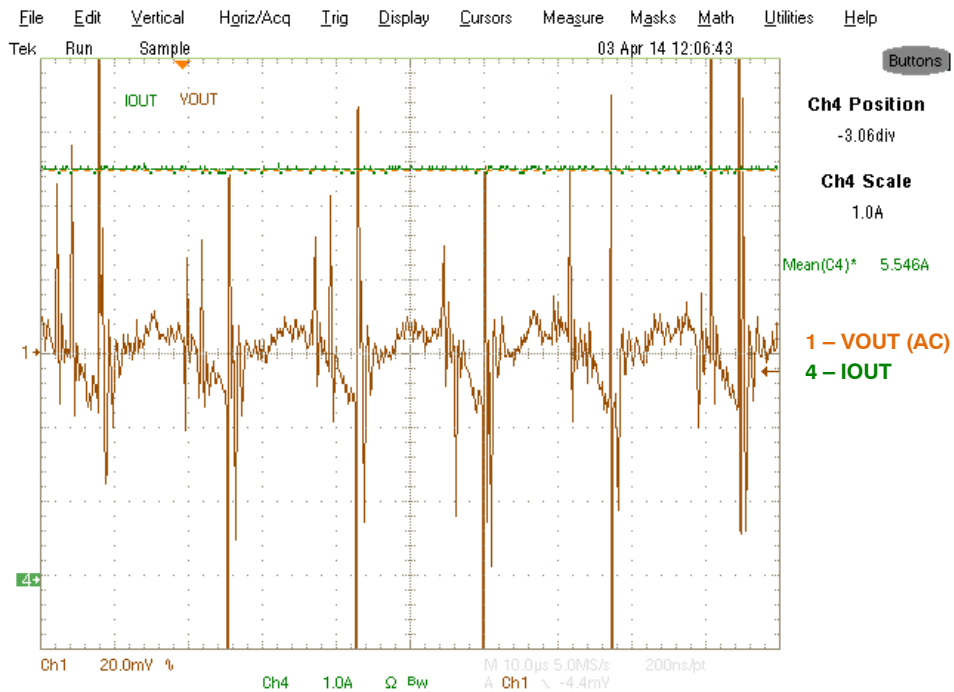
Figure 12. V_{IN} = 230 V_{AC} , I_{OUT} = 5.5 A , \Delta V_{OUTPK-PK} = 30 mV
