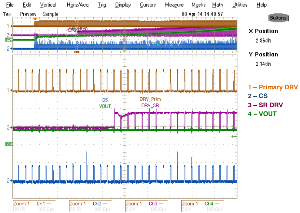
Figure 16. V_{IN} = 230 V_{AC} , I_{OUT} = 5.8 A , Start-up, SR Controller Starts to Operate Immediately after UVLO Level is Crossed
