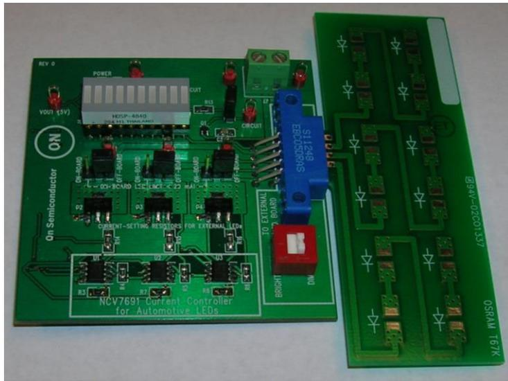
Figure 4. Load Board Interface with Controller Board
