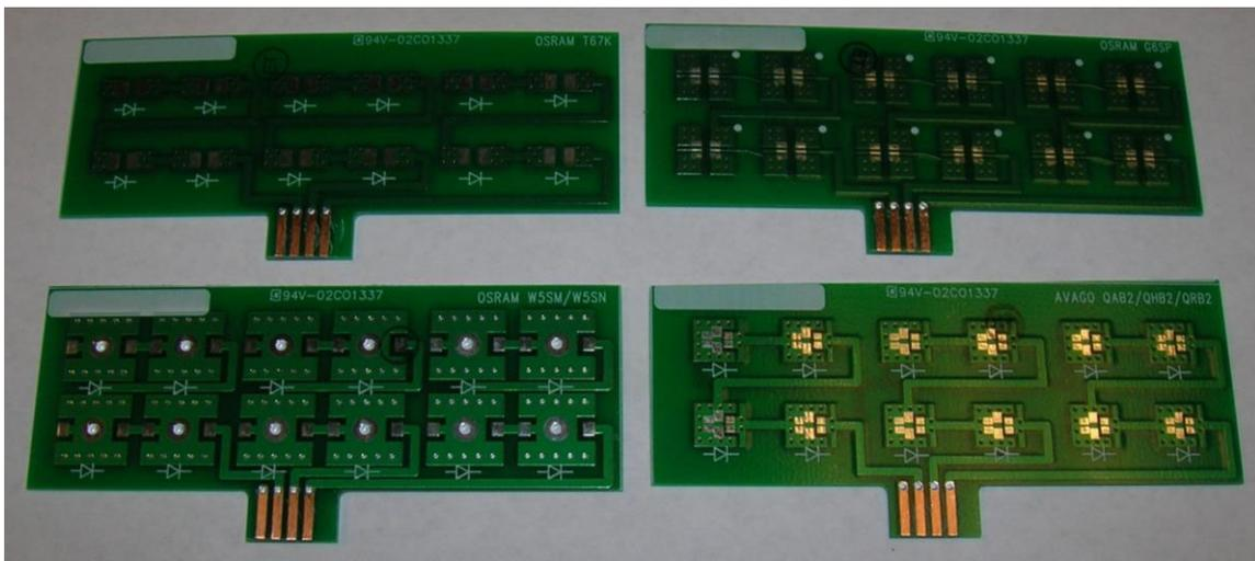
Figure 1. NCV7691 Optional External LED Load Boards
