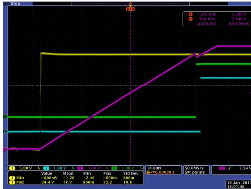
Figure 6. NCN5150 Startup Sequence
