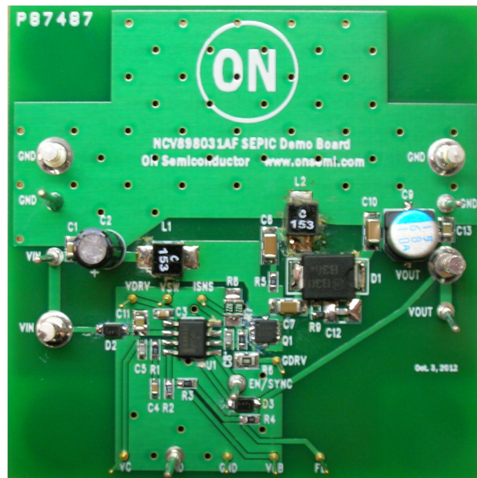
Figure 1. NCV898031 SEPIC Evaluation Board
