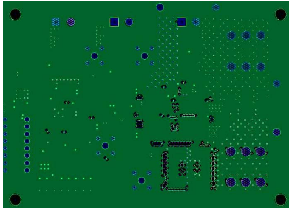
Figure 17. Internal Copper Layer 3 of ONS321G Evaluation Board
