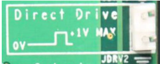
Figure 7. Direct Drive (Drives DLT Load Amps Directly)
