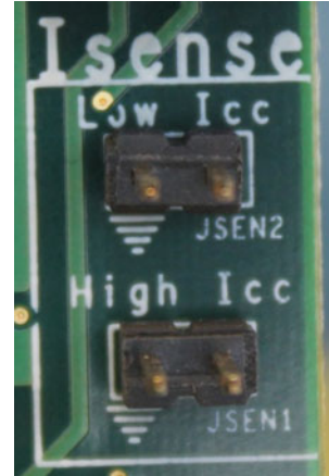
Figure 5. Current Monitor Sense Points
