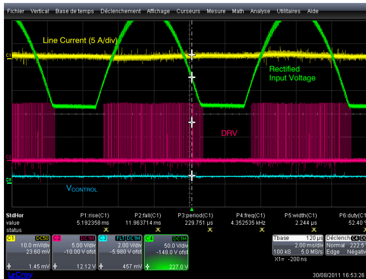
Figure 9. The Circuit Skips Cycle Near the Line Zero Crossing (265 V, 25% Load)
