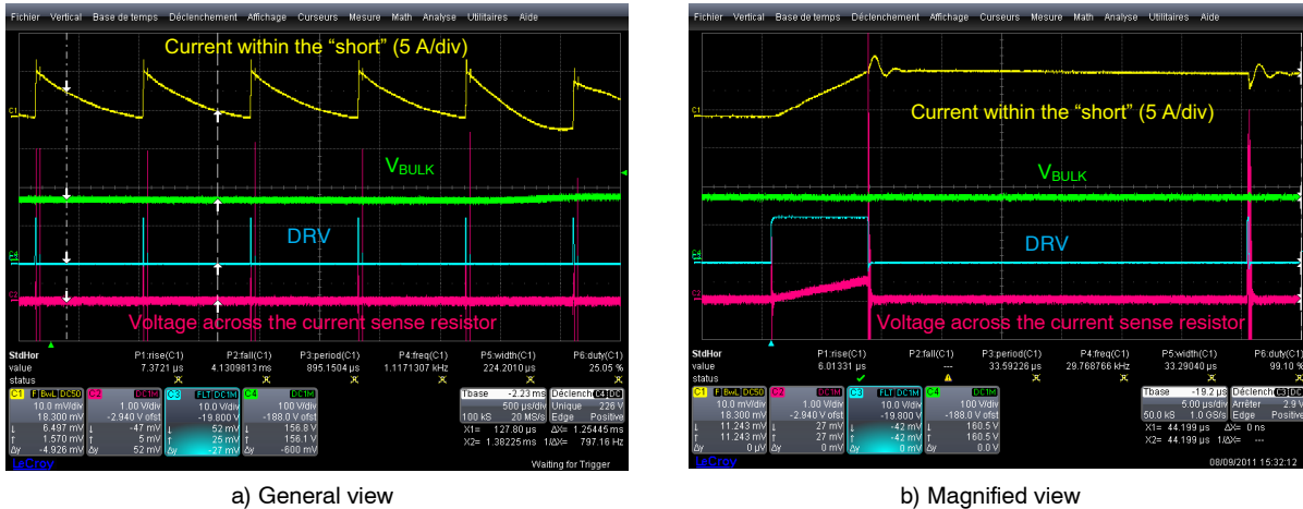
Figure 17. Shorting the Bypass Diode and the NTC
