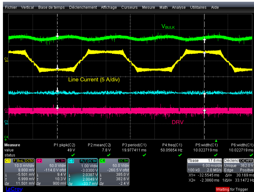
Figure 14. Over-Current Situation (85 V, 0.5 A Load Current)
