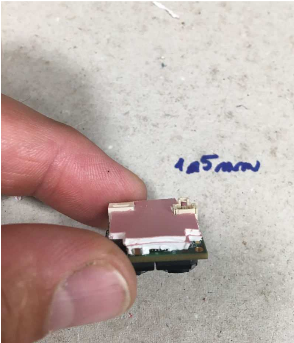
Both thermal pad cuts placement – side view
