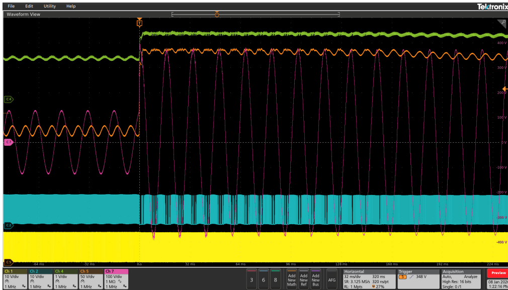
Figure 15. 90 Vac to 264 Vac Line Transition
