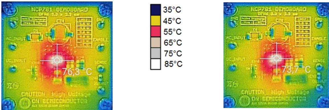
$V_{in} = 25\text{ V}$ ,  $P_d = 1\text{ W}$ ,
