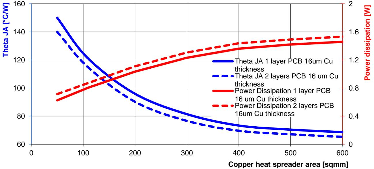
Figure 10. Maximum Power Dissipation &  $\theta_{JA}$  vs. Copper Area
