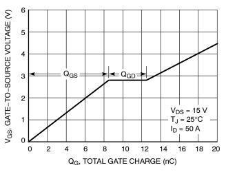
Figure 8. Gate-to-Source vs. Total Charge
