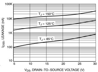
Figure 6. Drain-to-Source Leakage Current vs. Voltage
