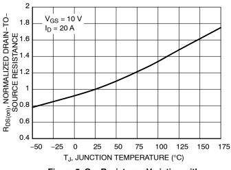
Figure 5. On–Resistance Variation with Temperature
