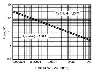
Figure 12. I<sub>PEAK</sub> vs. Time in Avalanche
