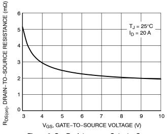
Figure 3. On-Resistance vs. Gate-to-Source Voltage
