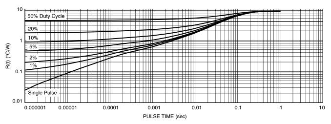
Figure 13. Thermal Characteristics
