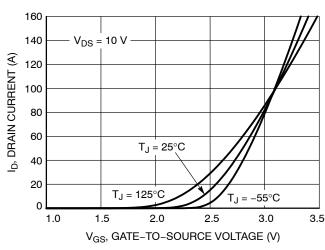
Figure 2. Transfer Characteristics
