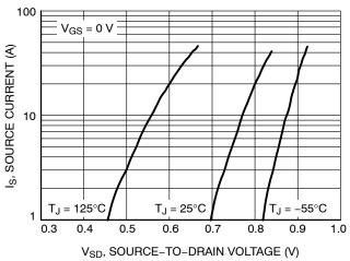
Figure 10. Diode Forward Voltage vs. Current
