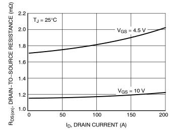
Figure 3. On-Resistance vs. Gate-to-Source Voltage
