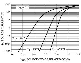
Figure 10. Diode Forward Voltage vs. Current
