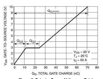
Figure 8. Gate-to-Source Voltage vs. Total Charge
