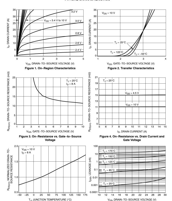
Figure 5. On–Resistance Variation with Temperature
