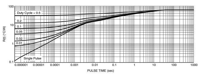
Figure 13. Transient Thermal Impedance
