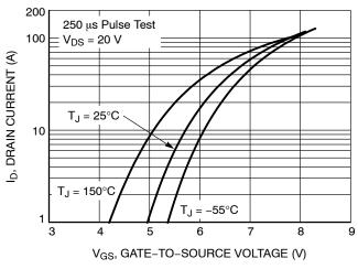
Figure 3. Transfer Characteristics
