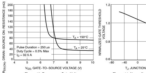
Figure 13. R<sub>DS(ON)</sub> vs. Gate Voltage
