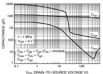
Figure 6. Capacitance Characteristics
