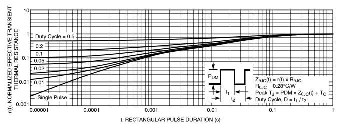
Figure 16. Transient Thermal Response Curve
