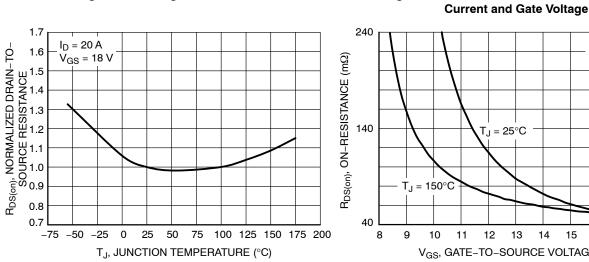
Figure 3. On-Resistance Variation with Temperature
