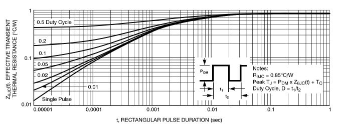
Figure 13. Junction-to-Case Thermal Response
