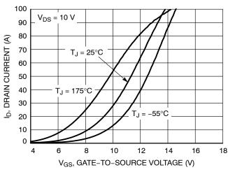
Figure 5. Transfer Characteristics
