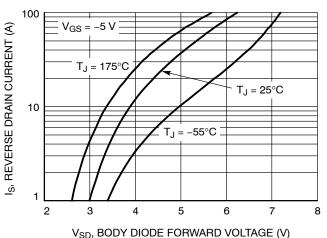
Figure 6. Diode Forward Voltage vs. Current
