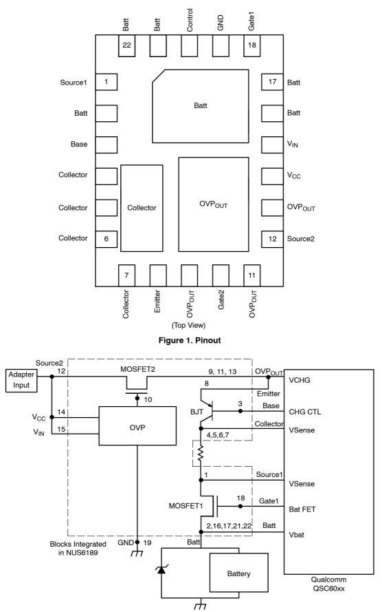
Figure 2. Typical Charging Solution for Qualcomm QSC60xx
