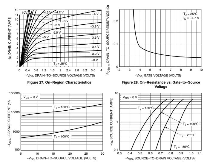
Figure 29. Drain-to-Source Leakage Current vs. Voltage
