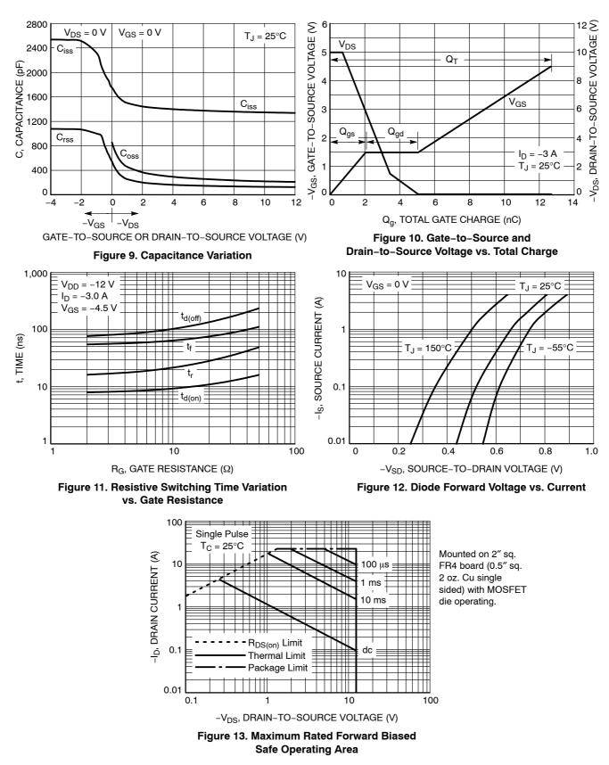
TYPICAL CHARACTERISTICS - 12V, P-CHANNEL MOSFETS (MOSFET1 - CHARGING)
