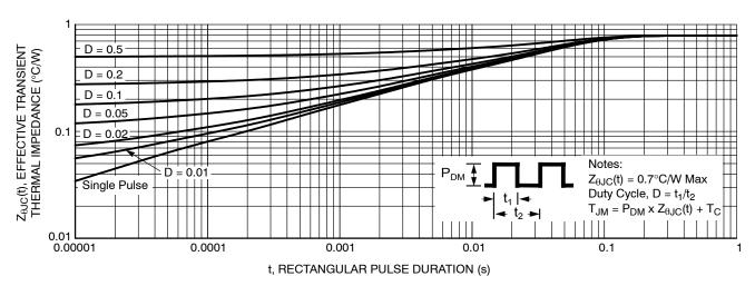
Figure 12. Transient Thermal Impedance
