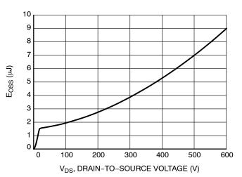
Figure 11. E<sub>OSS</sub> vs. Drain-to-Source Voltage
