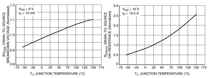
Figure 7. Breakdown Voltage Variation vs. Temperature
